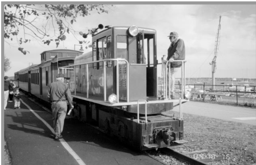
The power for the Maine Narrow Gauge Railroad's excursion train was this diminutive GE switcher. It is a very narrow locomotive. The body, minus the walkways, was only about 3 feet across. The consist included a caboose (restored Sandy River and Rangely Lake) and a coach. Portland, Maine, October 2004. digital image by Bob McCracken
