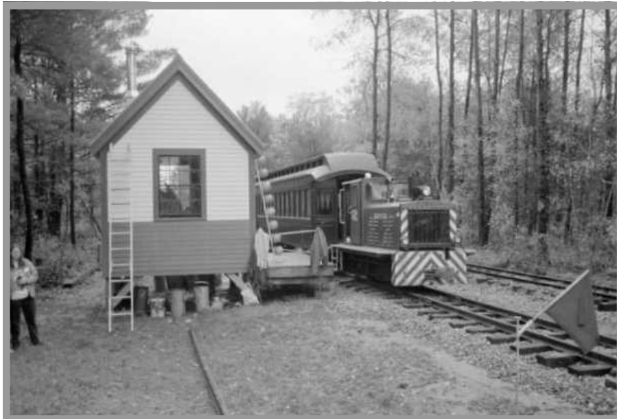
The Wiscasset, Waterville, and Farmington Railway operates on trackage that was once part of Maine's working 2 foot narrow gauge railroads. Power this day was a compact Plymouth gasoline locomotive. The coach is about 30' long, 7' wide and about 9' high. Even the depot has a narrow look. October 2004 digital image by Bob McCracken
