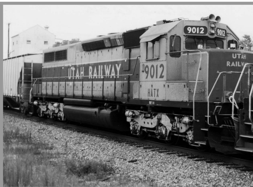
Among the seemingly endless variety of power in the CSX lease fleet is this unique SD45-2. It started life in 1972 as an ATSF unit, was repowered with a Caterpillar 4000 hp engine in 1987, then sold to Morrison Knudsen and leased to Utah Railway. It was returned to MK where it was reconfigured with it's original EMD 20-645ES engine and then all the MK units were sold to Helm. It was returned from Utah Railway in 2001 and now is working on CSX. She is seen here on CSX Q515 at 16th St. in Hopkinsville on October 10, 2004, still in Utah Railway paint. Color print by Wallace Henderson
